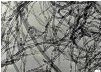
TEM, 10-20 nm grade (030203, ID 252). Scale bar 100 nm.
