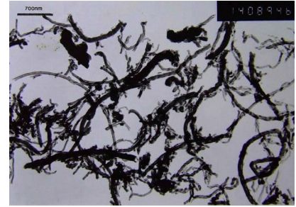
TEM, short pristine 50-80 nm (030407, ID 215). Scale bar 700 nm.
