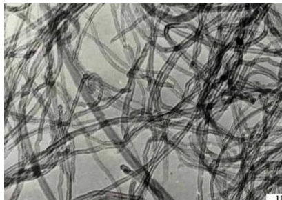
TEM, 10-20 nm grade (030103, ID 171). Scale bar 100 nm.
