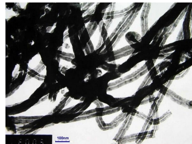
TEM, 50-80 nm grade (030107, ID 178). Scale bar 100 nm.
